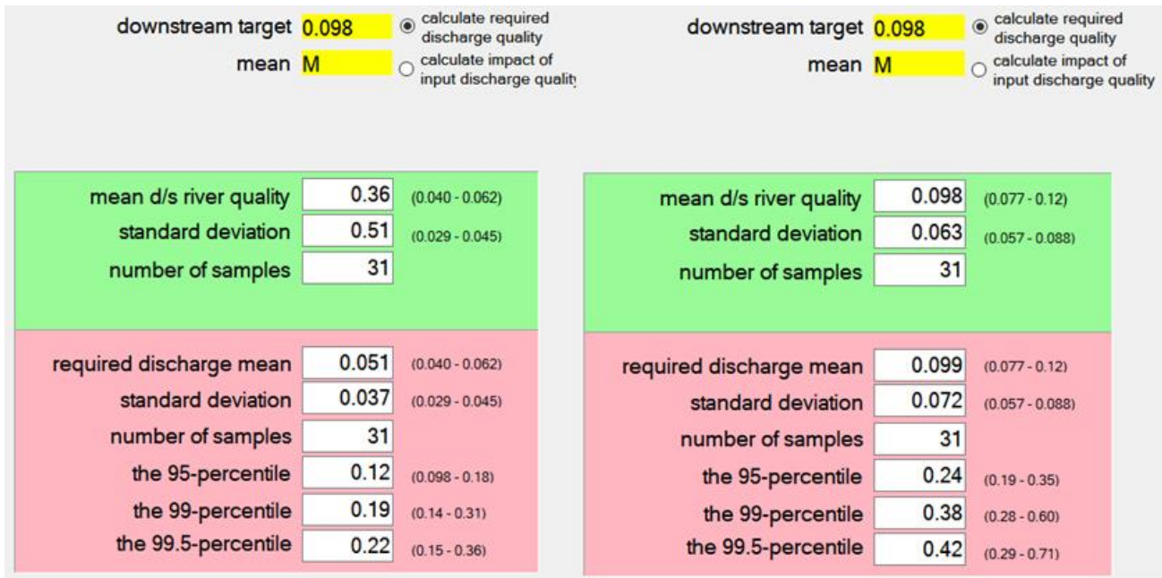
Figure 9-3: RQP required to meet no deterioration results for mancozeb (continuous and intermittent flows, left, continuous only flows, right).
