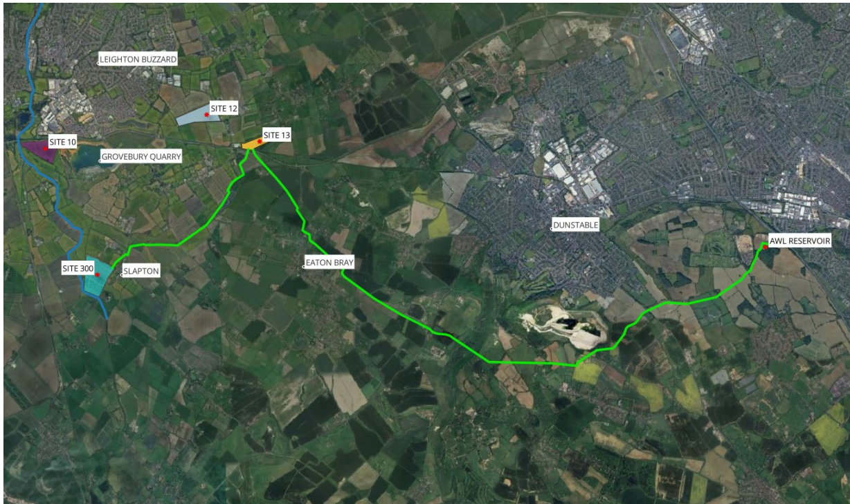
Figure 11-10 Current Possible Route Corridor for Pipeline Site Q Potable from Site Q to AfW Service Reservoir
