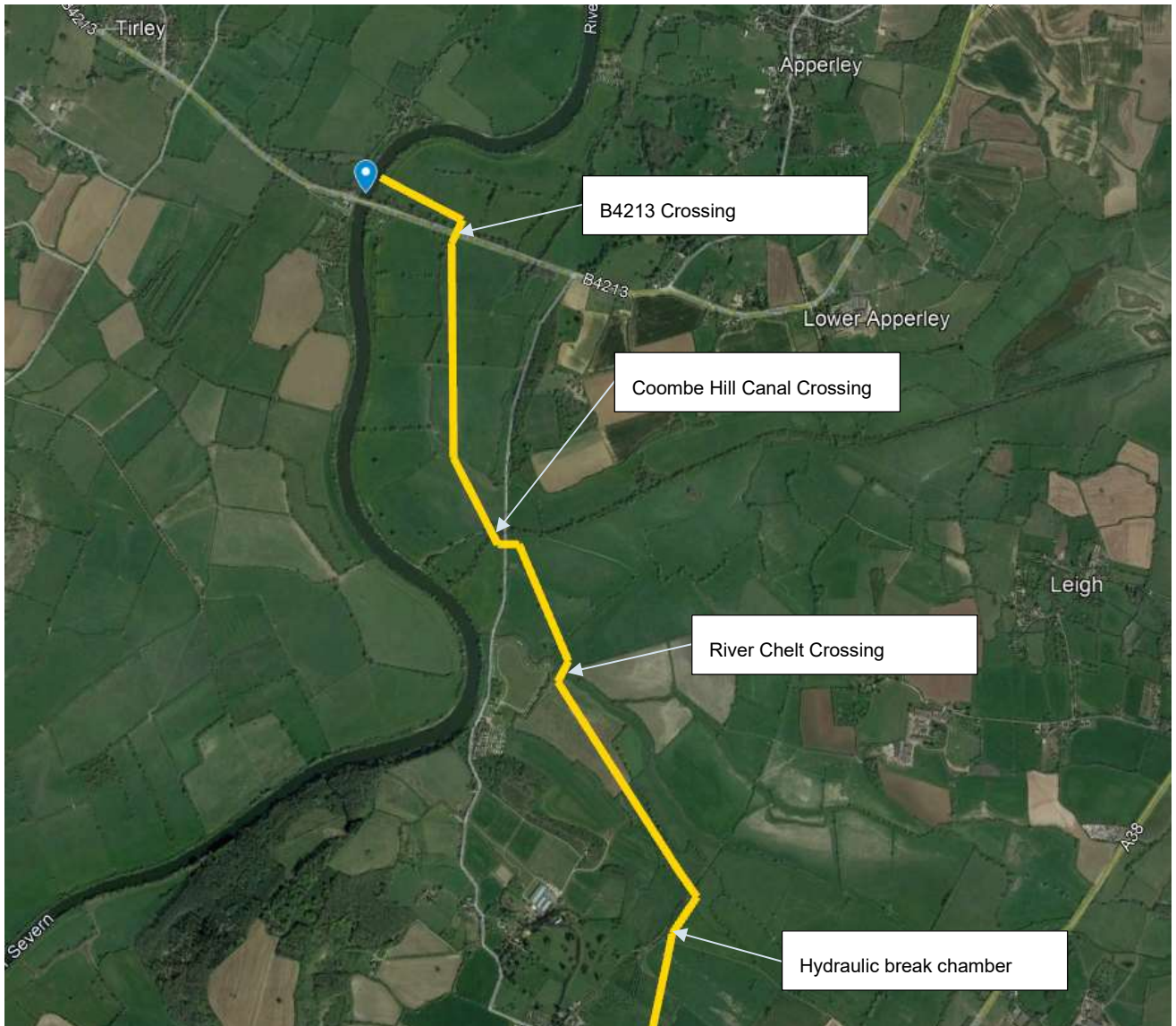
Figure 4-8 – Option 2 – Generalised route to Haw Bridge
