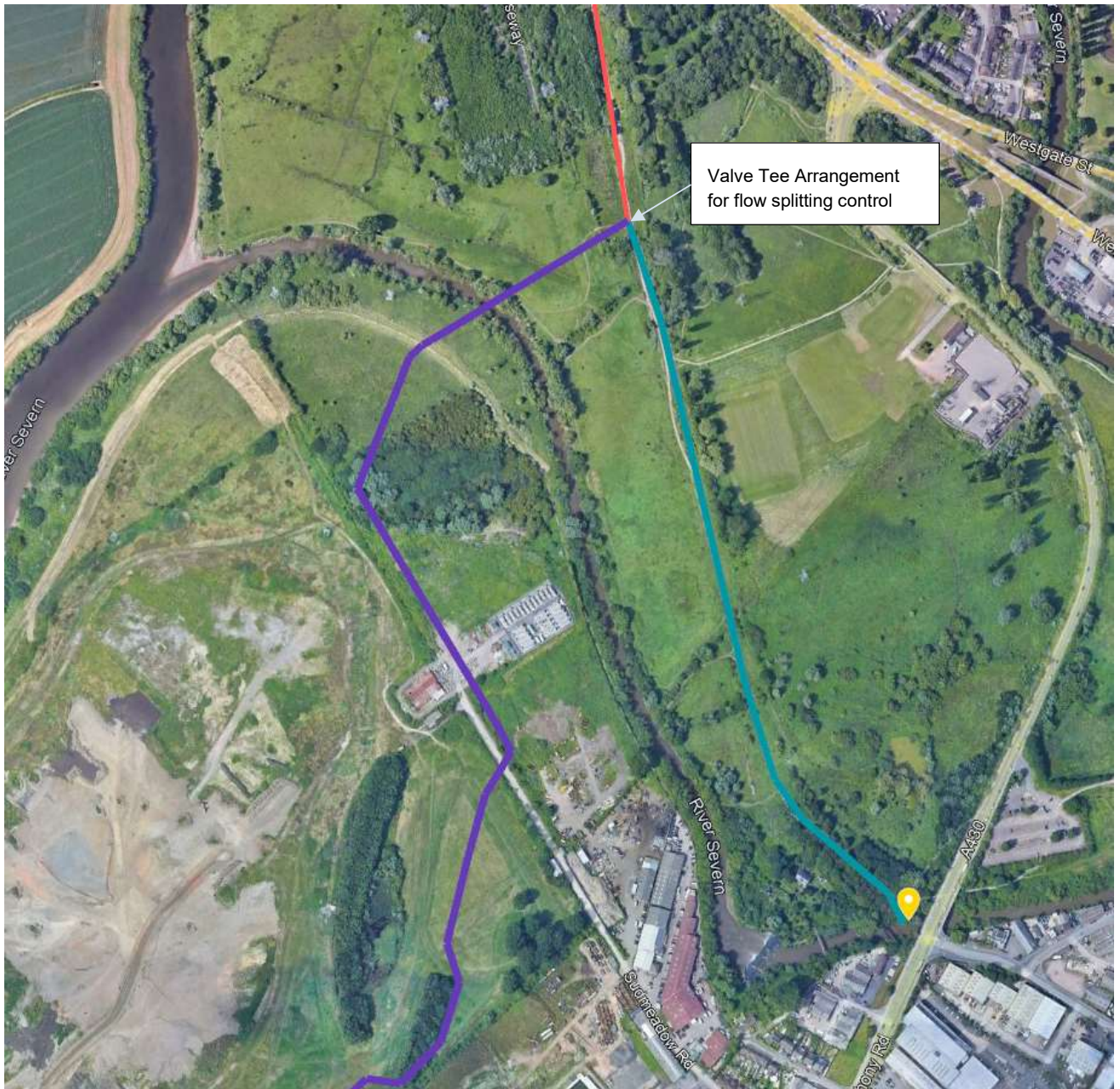
Figure 4-11 – Flow Splitting Location to Enable Option 5
