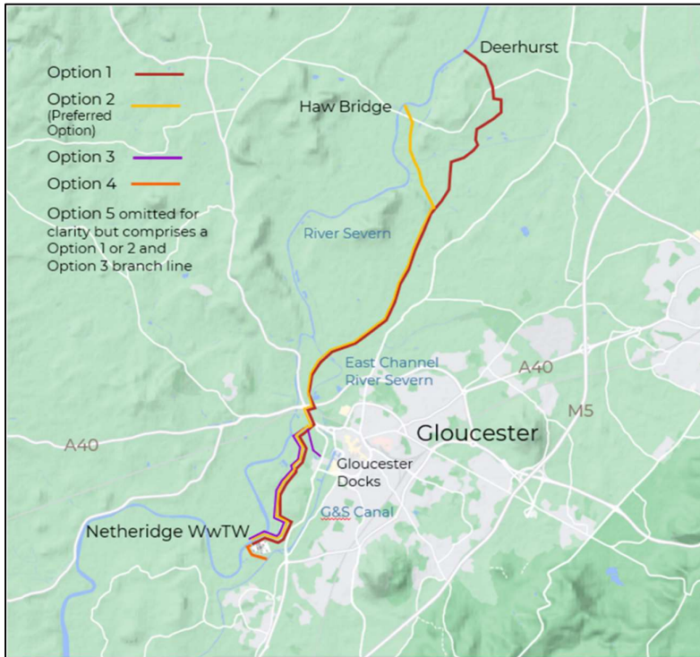
Figure 1-2: STS SRO pipeline route
