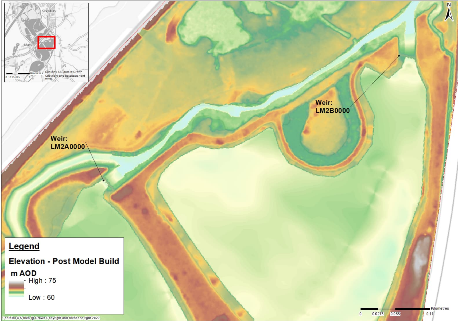
Figure 2-10: River Tame at Lea Marston – Topographic Elevation Post Model Build, weirs LM2A0000 & LM2B0000
