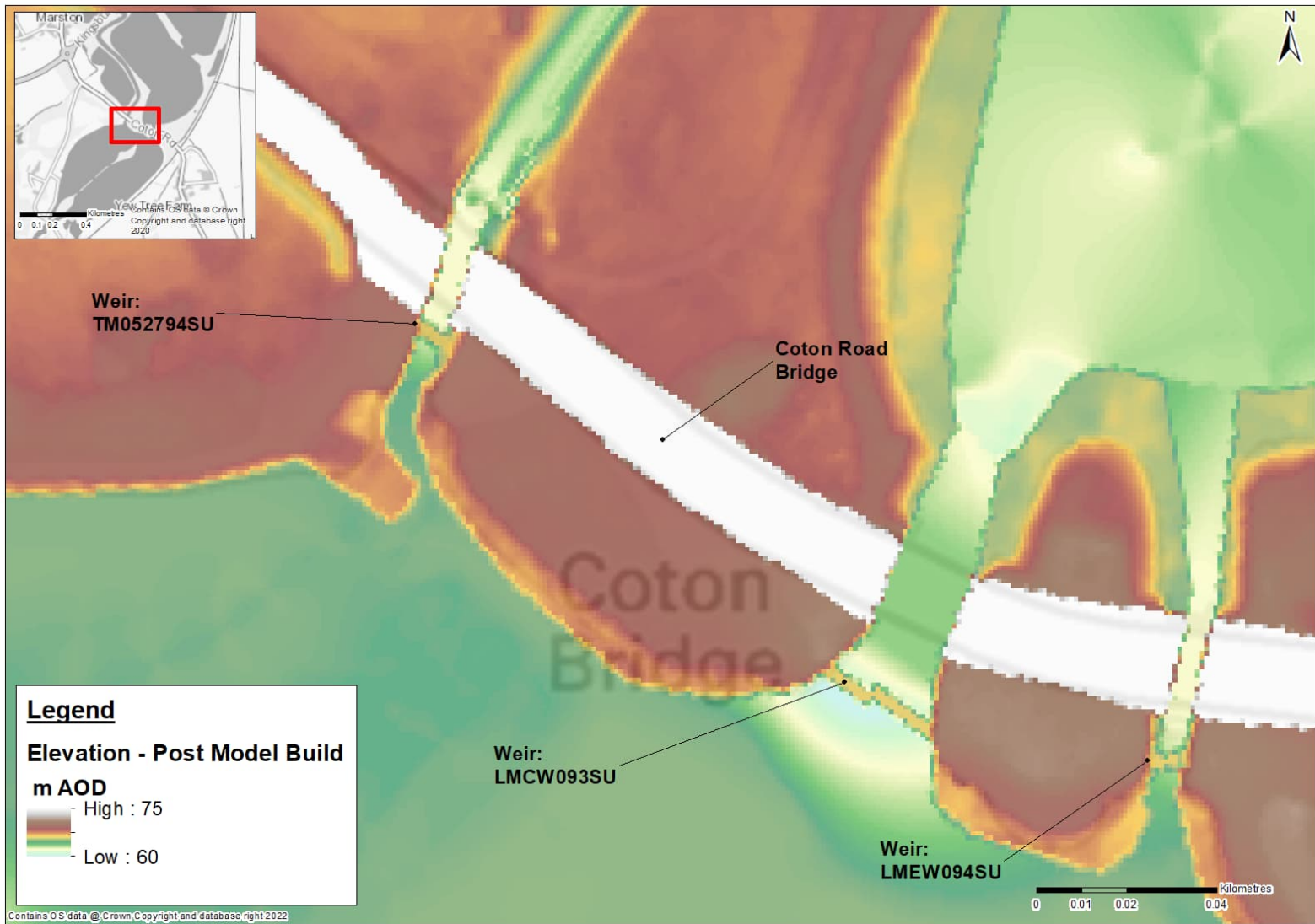
Figure 2-8: River Tame at Lea Marston – Topographic Elevation Post Model, Cotton Road Weirs TM052794SU, LMCW093SU & LMEW094SU
