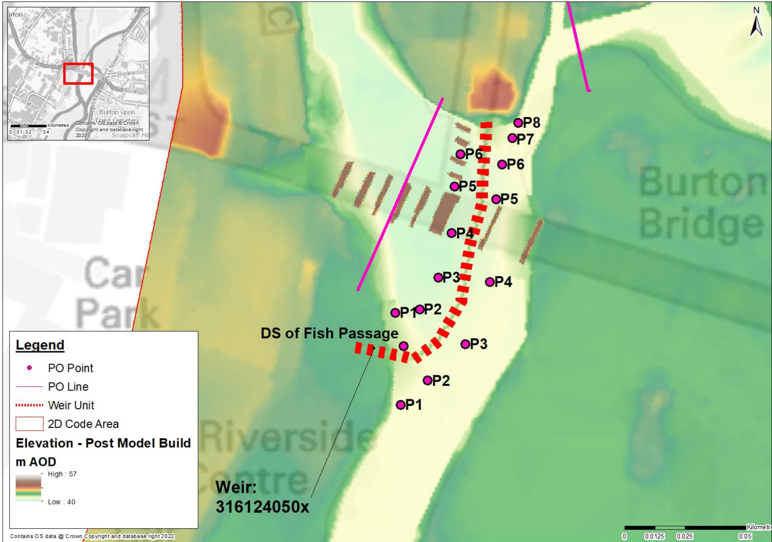
Figure 3-23: River Trent at Winshill – PO Points & Lines at Weir No.1, 316124050x
