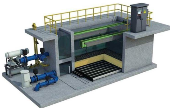
Figure 2-5: BAC Filtration Treatment cell (courtesy of Xylem-Leopold)
