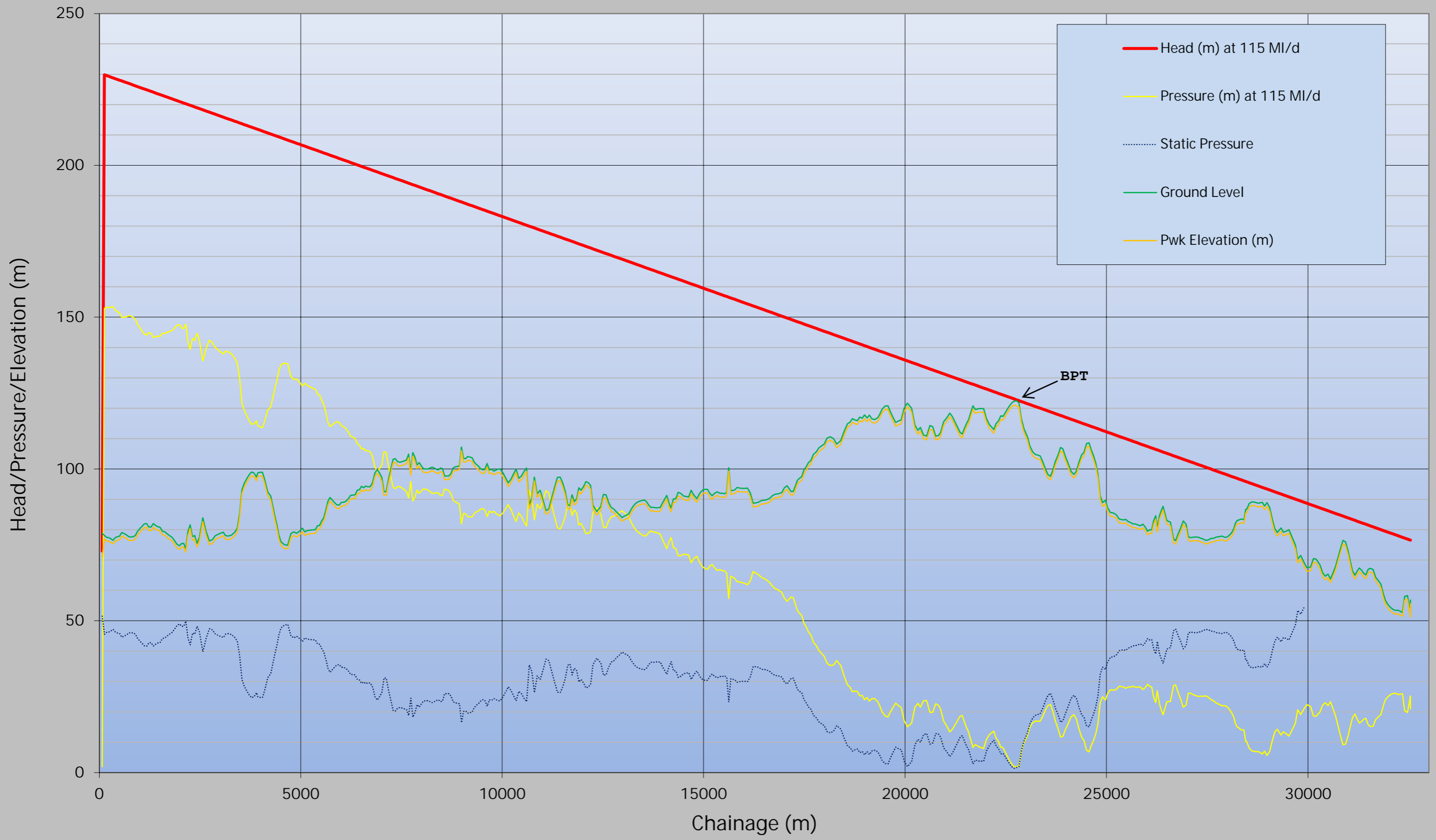
Profile of Gate 1 North Warwick - 1No. 900mm Rising Main followed by 1No. 900mm Gravity Main
