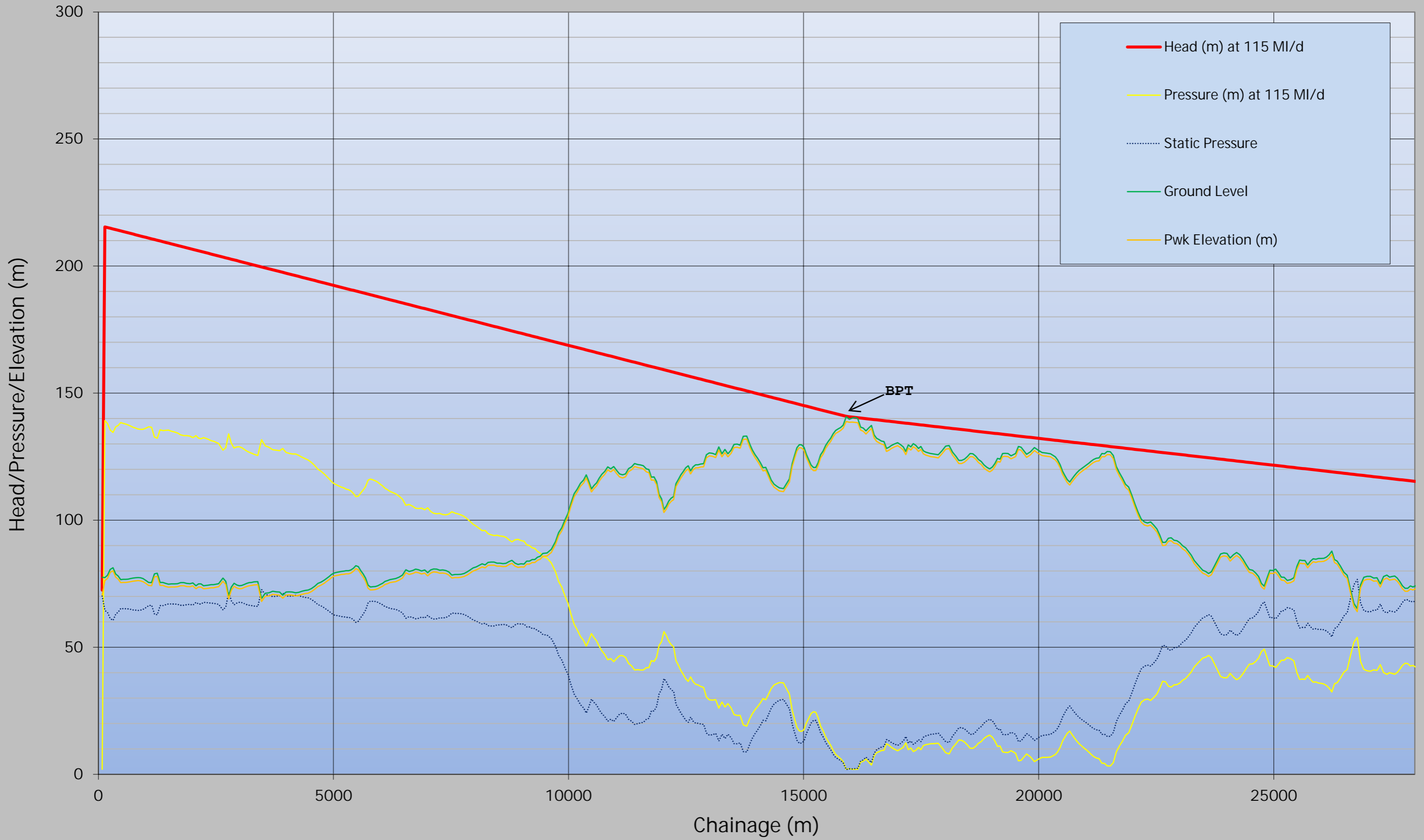
Profile of Gate 2 WRMP19 - 1No. 900mm Rising Main followed by 1No. 1050mm Gravity Main
