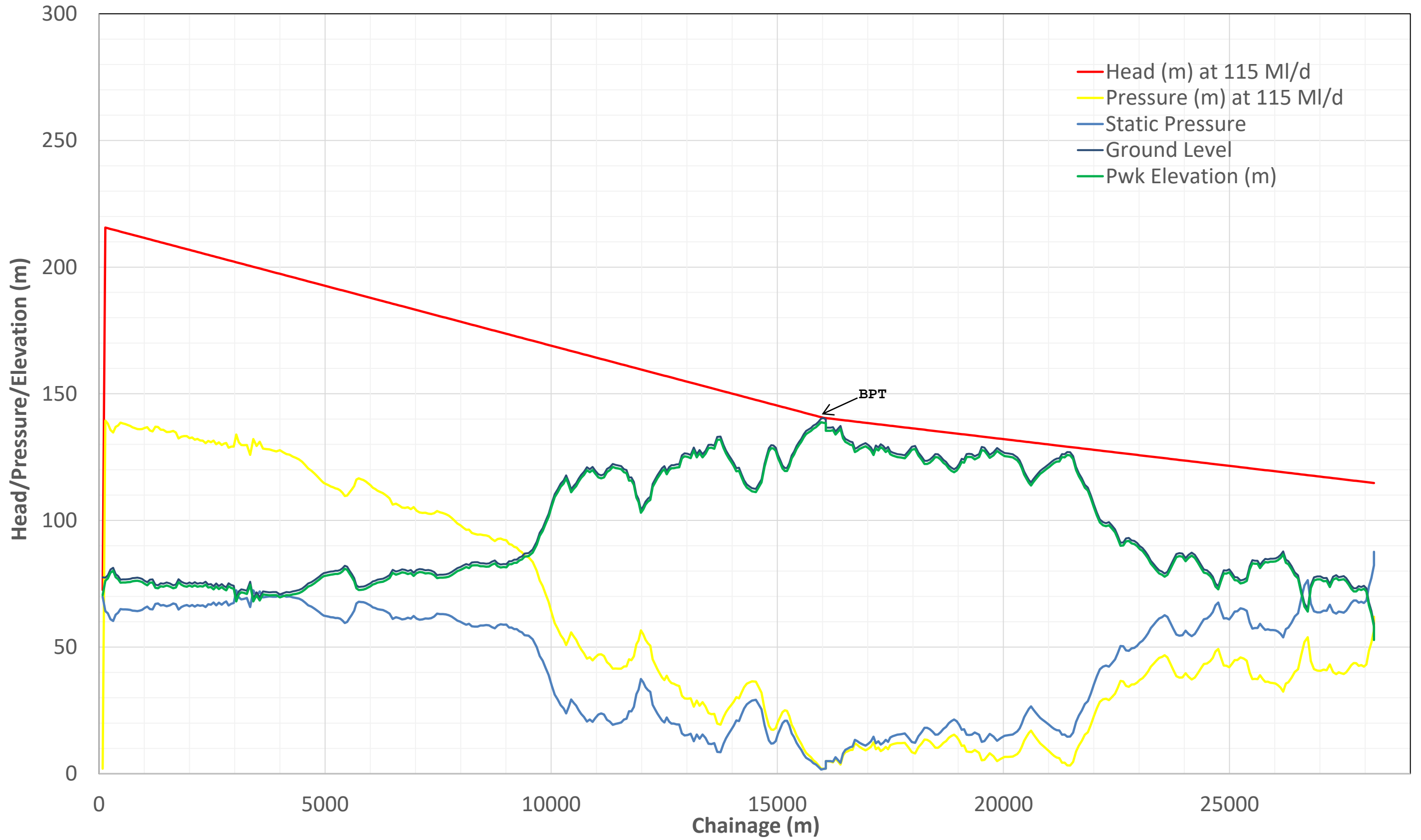
Profile of Gate 2 WRMP19 RE_A Route - 1No. 900mm Rising Main followed by 1No. 1050mm Gravity Main
