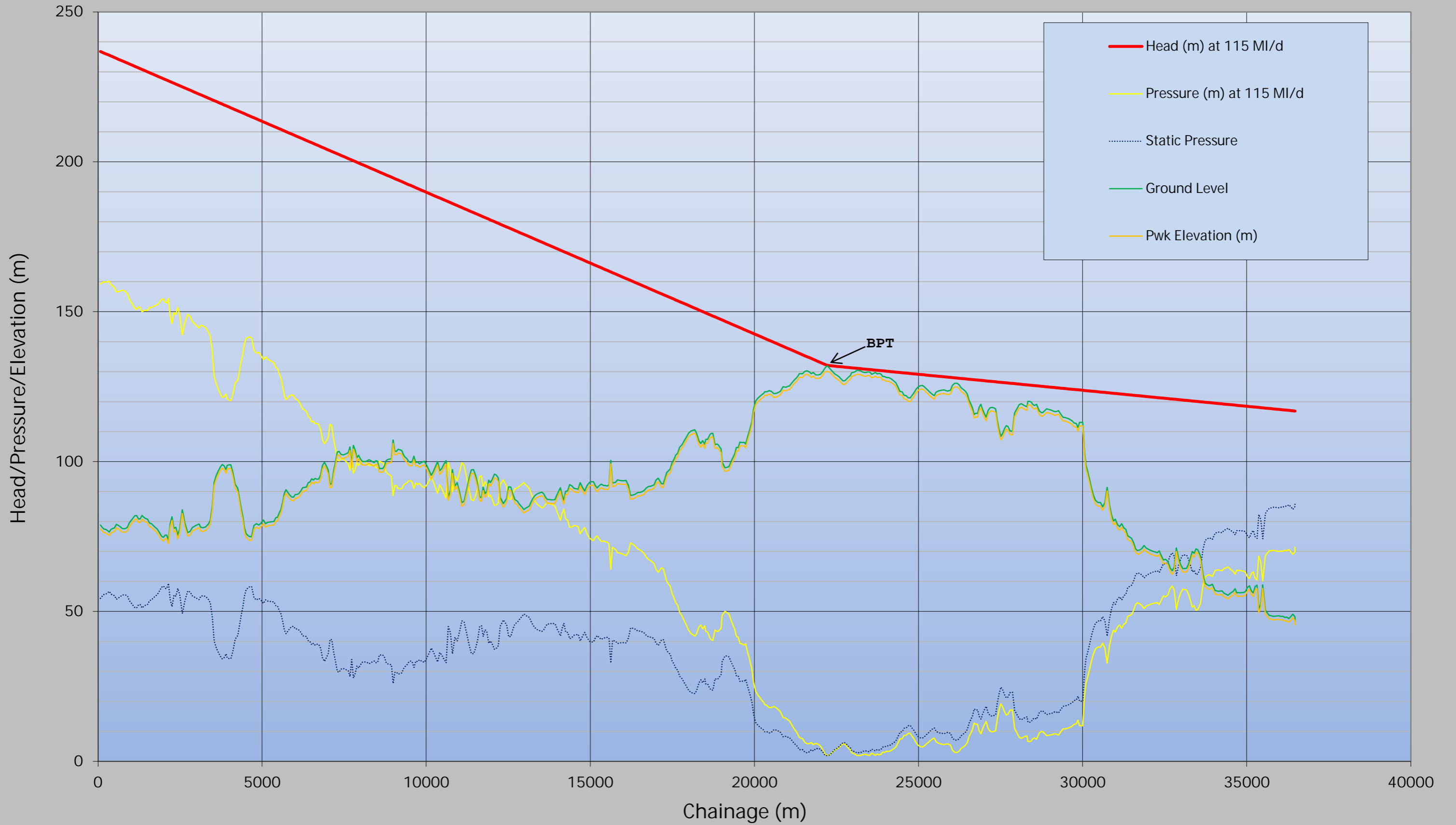
Profile of Gate 1 South Warwick - 1No. 900mm Rising Main followed by 1No. 1200mm Gravity Main
