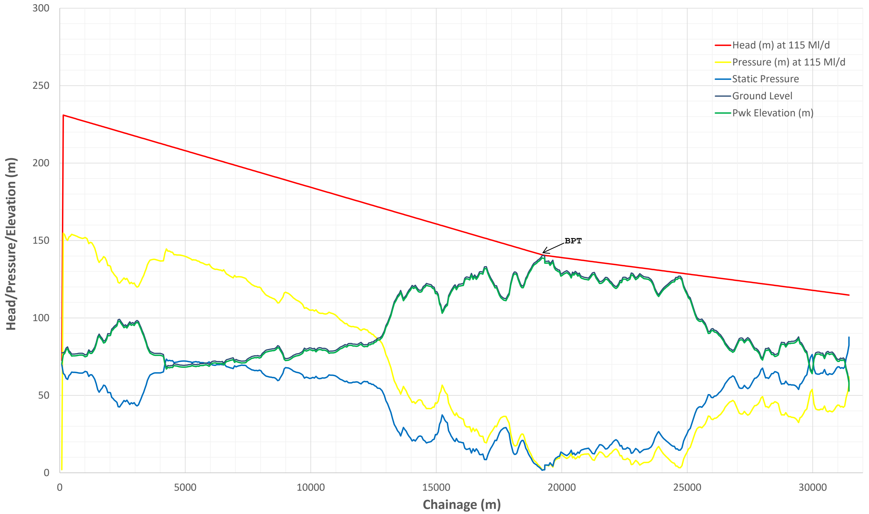
Profile of Gate 2 WRMP19 RE_B Route - 1No. 900mm Rising Main followed by 1No. 1050mm Gravity Main
