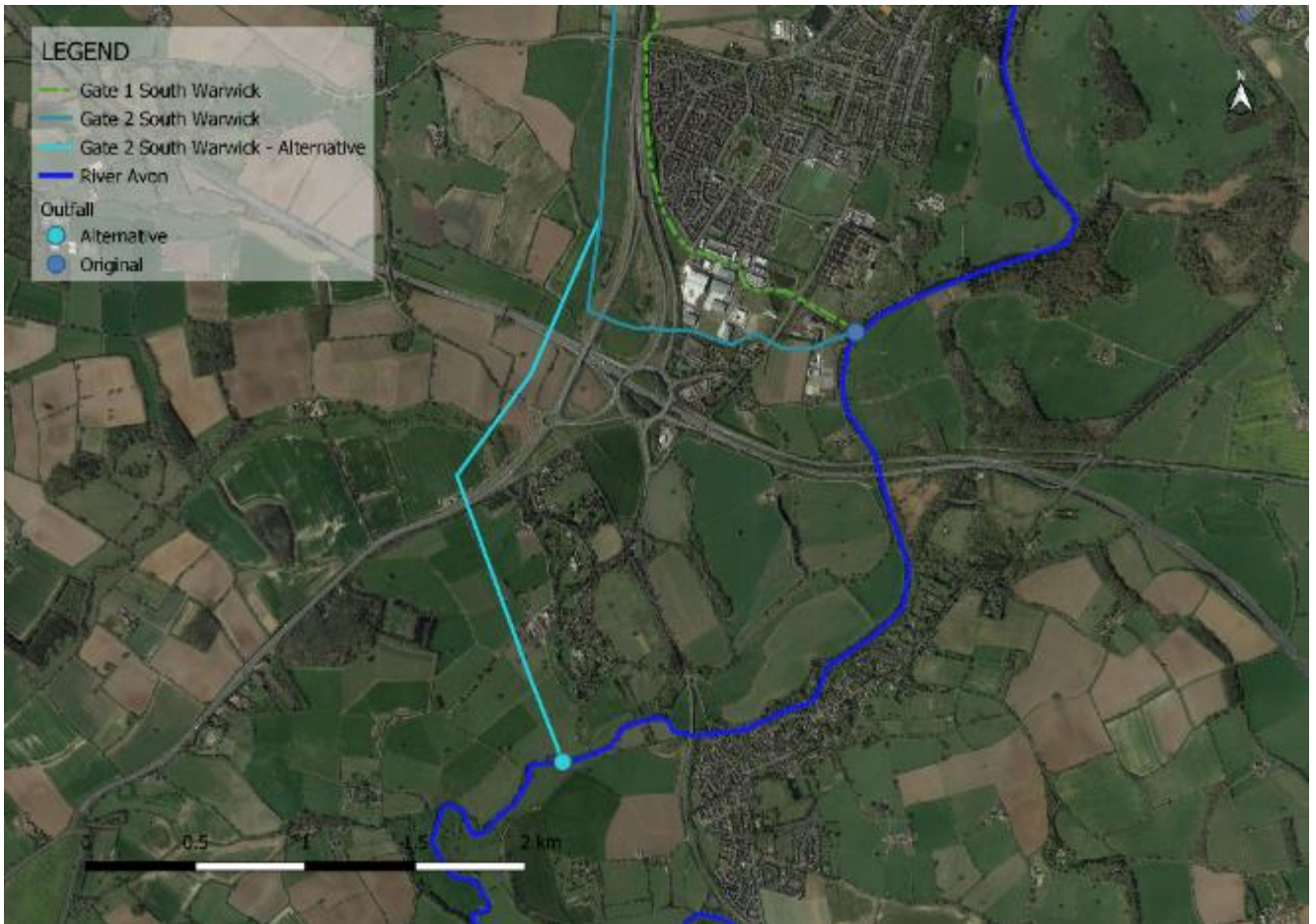
Figure 6-2: Opportunity for alternative outfall location at South Warwick to avoid built-up area crossings
