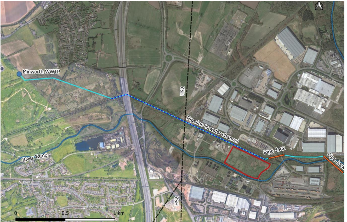
Figure 6-5: Route G2 WRMP19 RE_A modified route to pass along the length of the discharge channel
