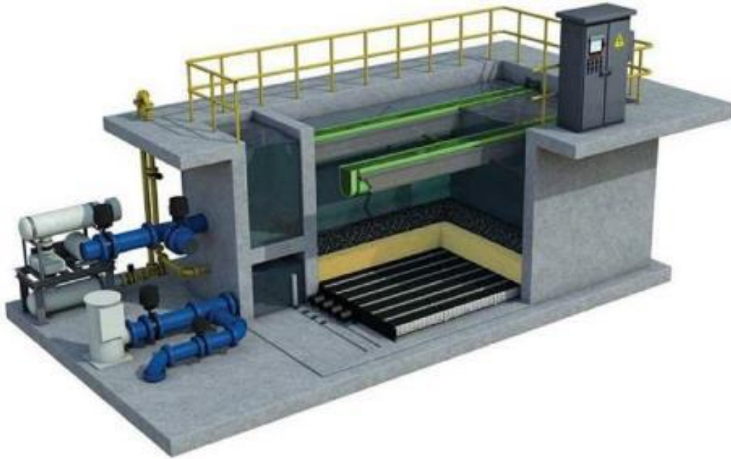
Figure 2-5: GAC Adsorption Treatment Cell (courtesy of Xylem-Leopold)
