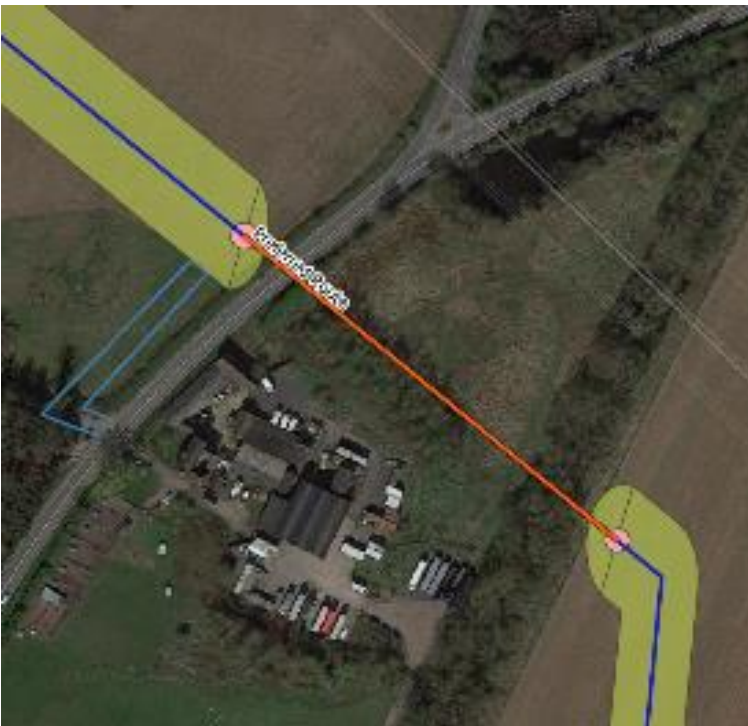
Figure 3-4: Example of additional working room required around the perimeter of a shaft.
