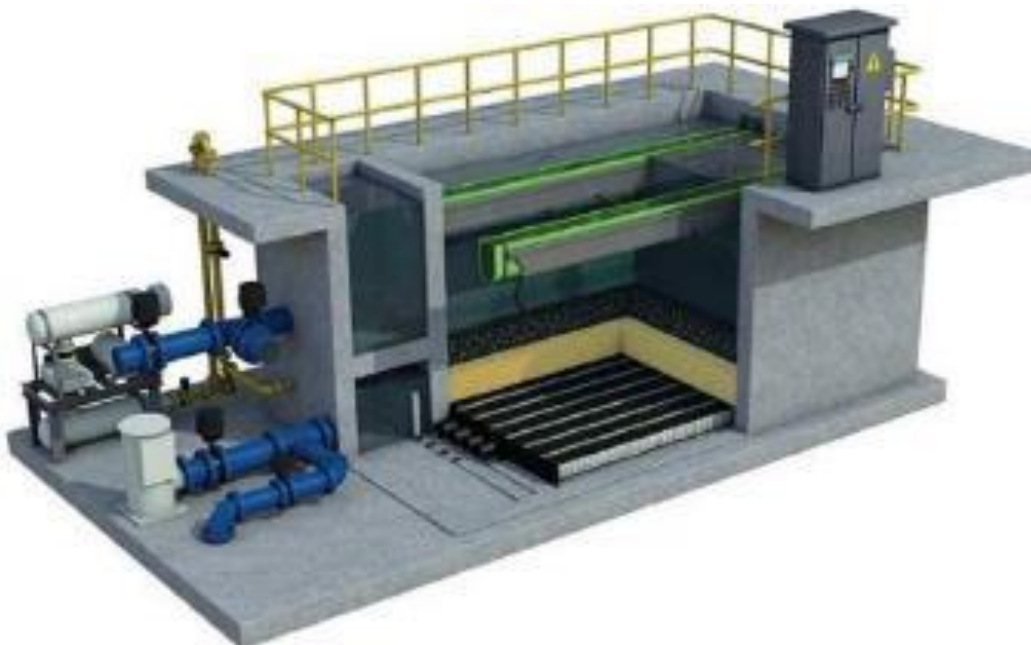
Figure 2-4: BAC Filtration Treatment cell (courtesy of Xylem-Leopold)
