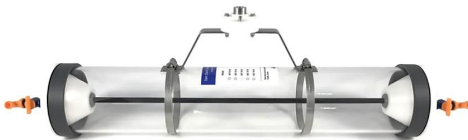
Figure 2.7: Van Dorn water sampler comprising a falling weight (messenger), horizontal water bottle, and rope.
