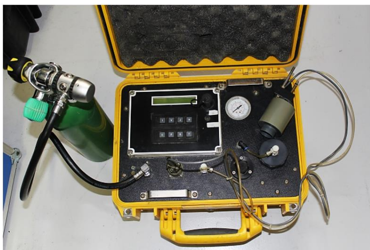
Figure 2.9: CSM; the portable instrument used to measure the critical entrainment stress of canal bed and connected waterbody sediments.
