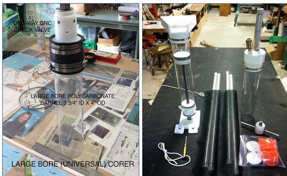
Figure 2.3: Large-bore sediment sampler unit supplied by Aquatic Research Instruments used to obtain bottom sediment samples.
