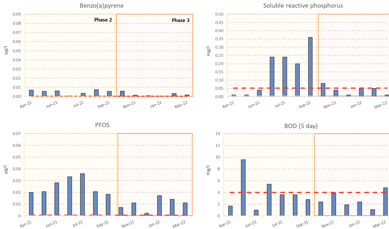
Figure 3-7 - Spatial trends in for key determinands at Site 5 GUC at Welton Lane, Daventry (April 2021 - March 2022) 37 .
