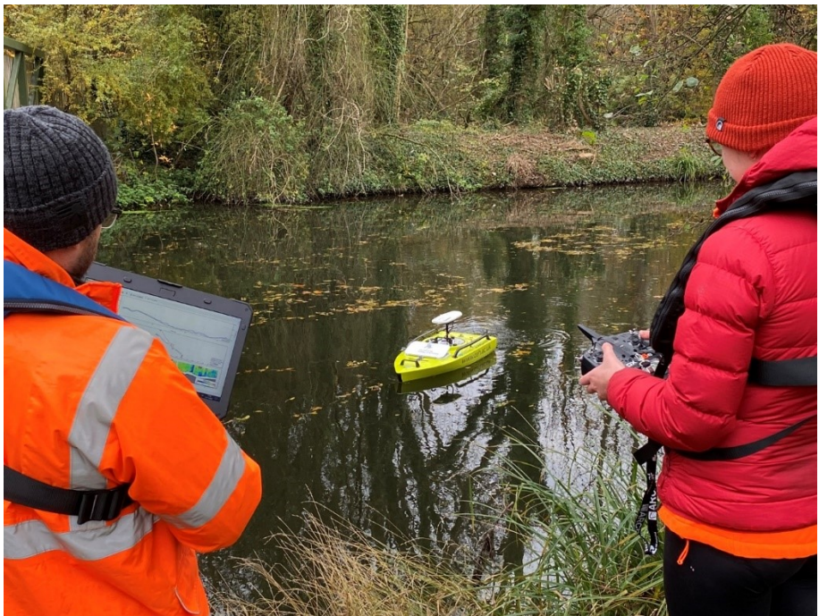
Figure 4-3: Flow gauging using the Acoustic Doppler Current Profiler mounted to a remote-controlled boat
