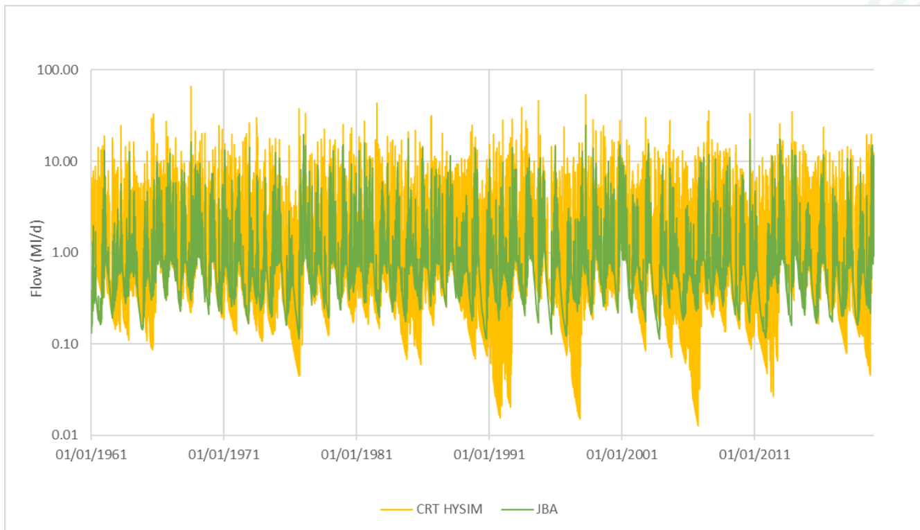
Figure 4-14; Comparison of Trust and JBA Aquator model inflows for the Drayton Feeder
