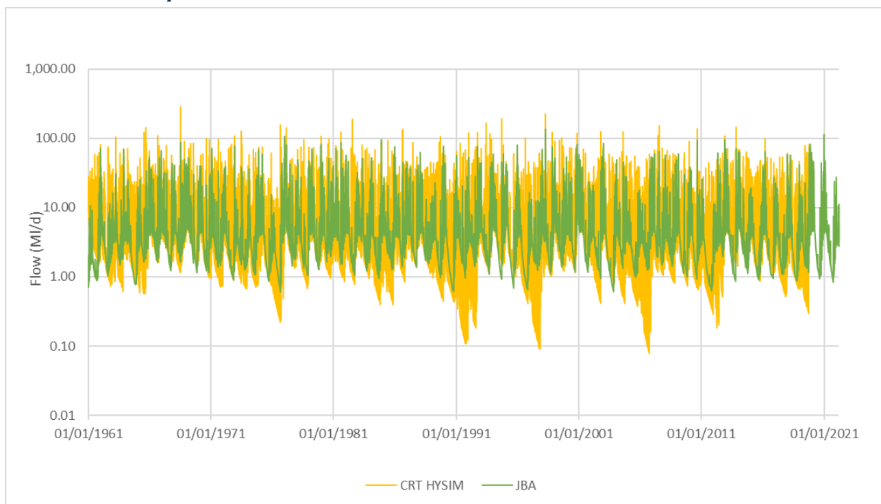
Figure 4-16; Comparison of Trust and JBA Aquator model inflows for the Daventry Feeder
