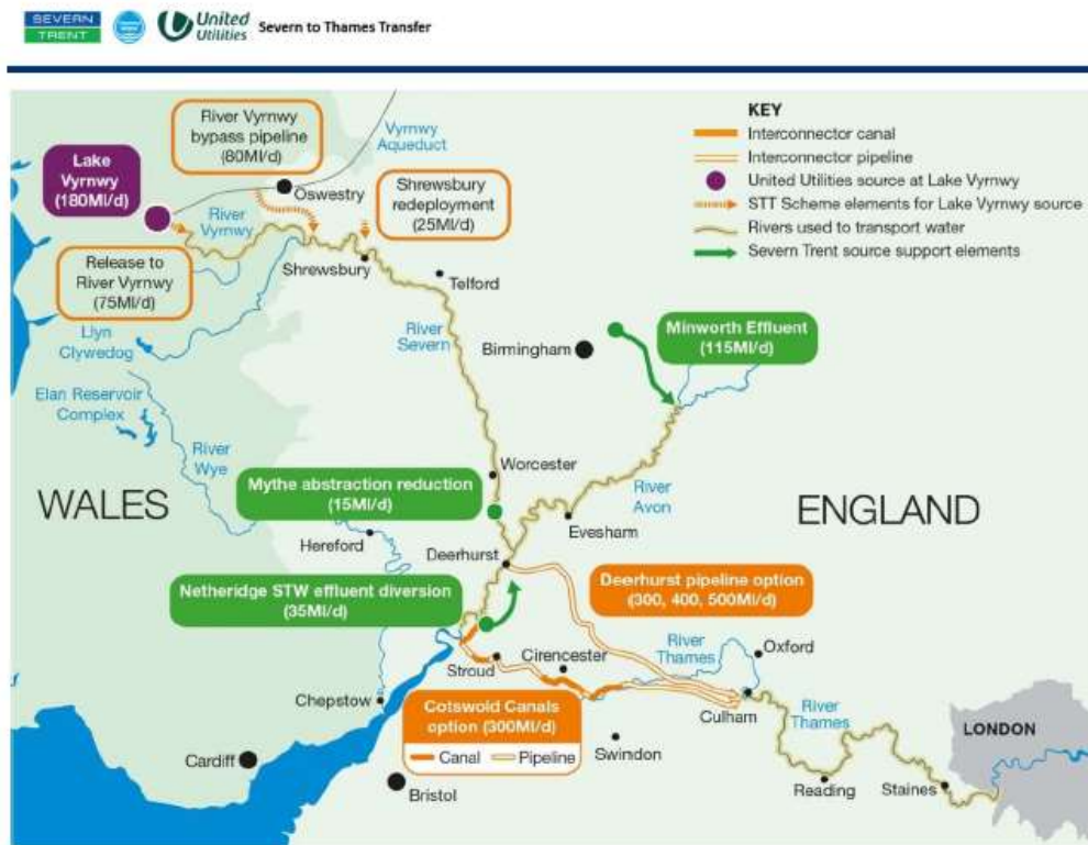
Figure E5.1: The Severn to Thames Transfer scheme
